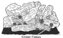
Figure 27 - Installing Ember Flakes
